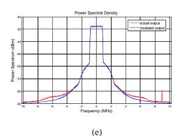
Fig. 2: Power spectral density (PSD) of actual and modeled PA showed for: (a) Q=2, K=3, (b) Q=2, K=5, (c) Q=3, K=2, (d) Q=3, K=5 and (e) Q=5, K=5.
