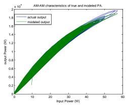
Fig.1: Comparison of AM/AM characteristics of actual and modeled PA
